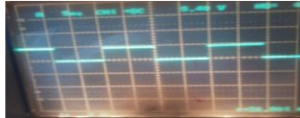
Fig 10 (b). current signal after passing through the zero crossing detector
