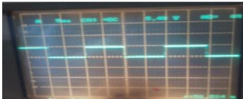
Fig 10 (a). Voltage signal after passing through the zero crossing detector
