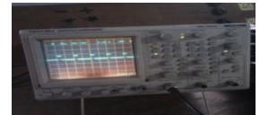
Fig 11. The output signal for Exclusive-OR gate
