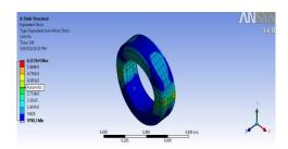
Fig 7. von-Mises-Hencky stresses for vertical loading
