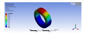
Fig 5. Tire Deformation under Vertical Load
