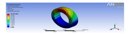
Fig 4. Total deformation of inflated tire
