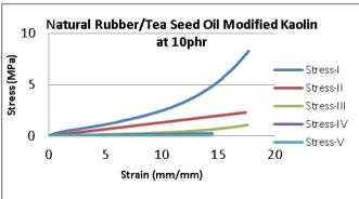
Fig 1. Stress-Strain plot of Natural Rubber/Tea Seed Oil modified Kaolin composites at 10phr
